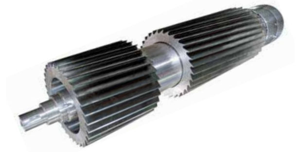
Scheer rotor with 200 mm diameter
